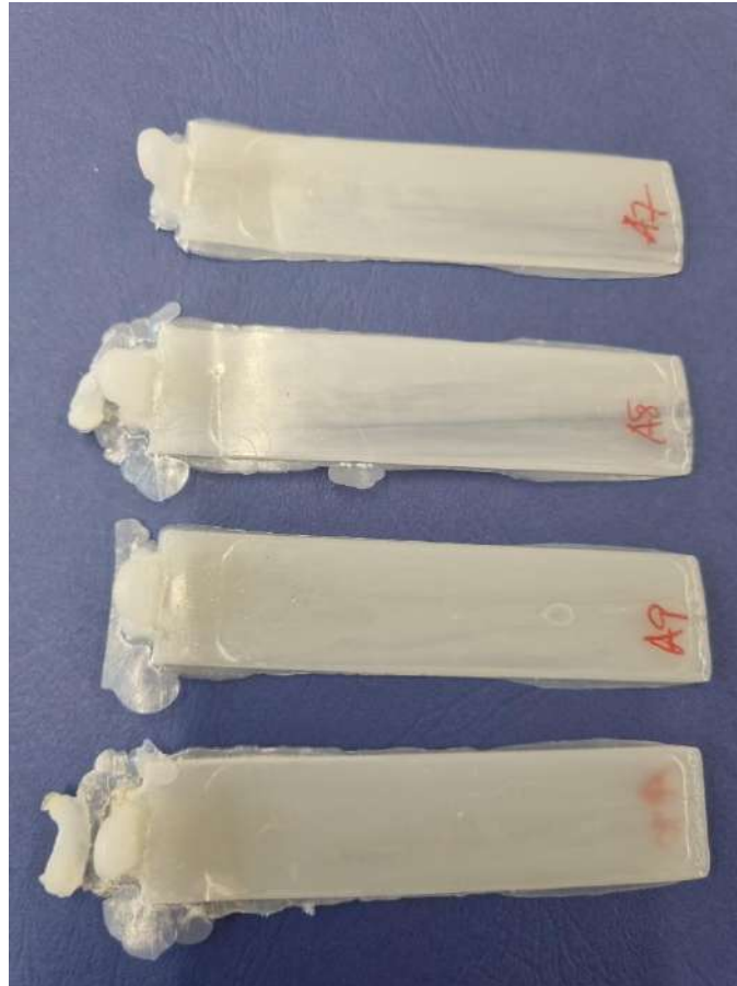
Figure 7 Photographs of the parts produced by injection moulding runs 7,8,9,10, 7 at top 10 at bottom (see Table 2)
