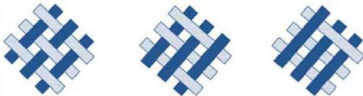
Diamond Braid (1/1) Regular Braid (2/2) Hercules Braid (3/3)
