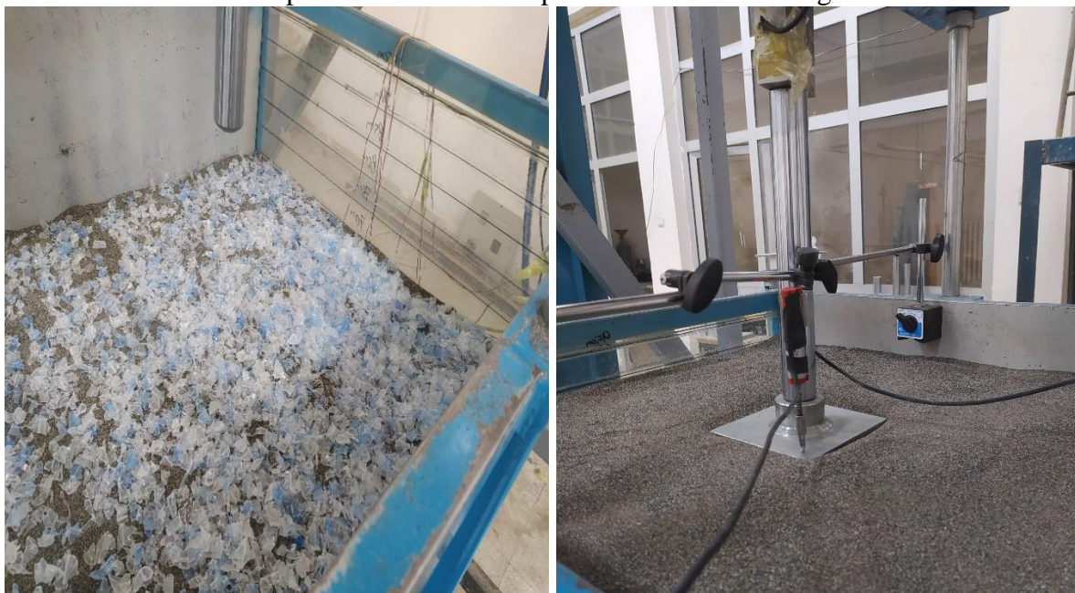
Figure 3. Experimental study (a) Randomly distributed PET waste (b) Loading system
