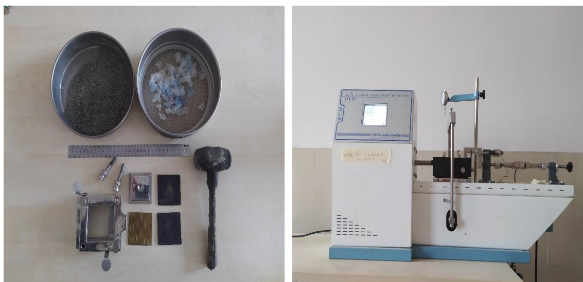
Figure 2. Preparation for direct shear test and experimentation
