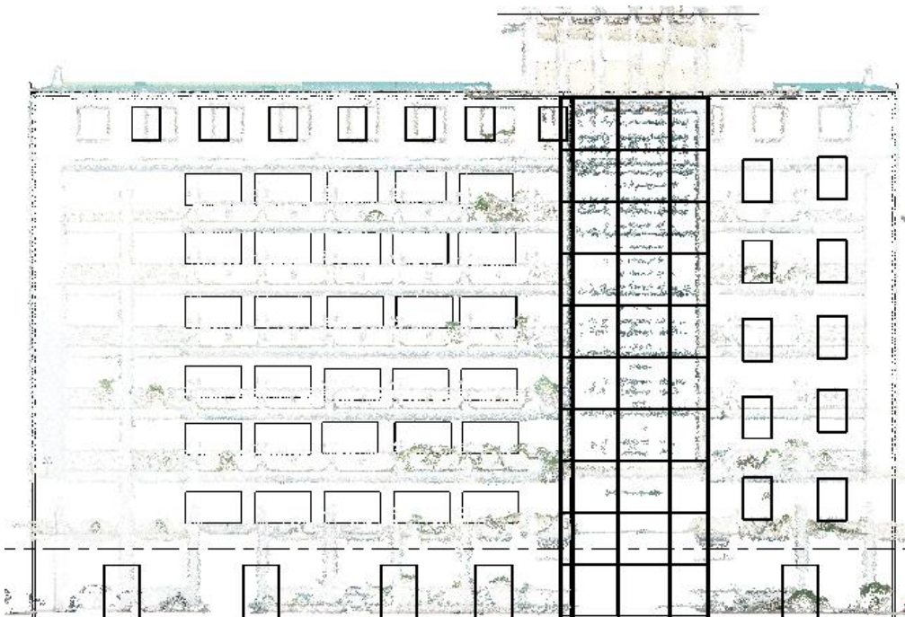
Figure 3. The shape of the point cloud of a building after processing
