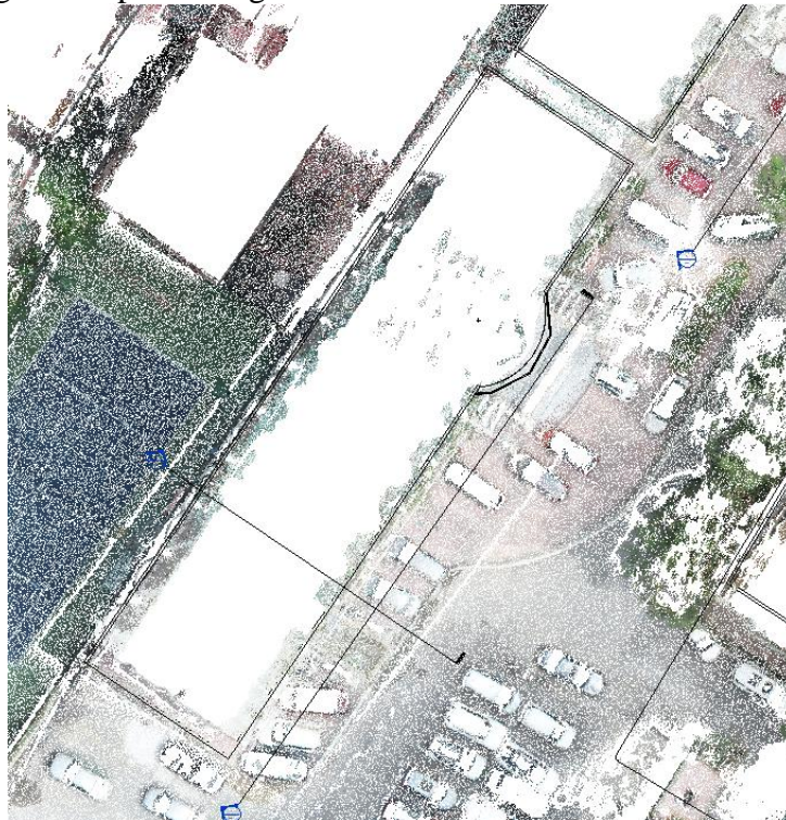
Figure 2. The shape of the point cloud of a building before processing
