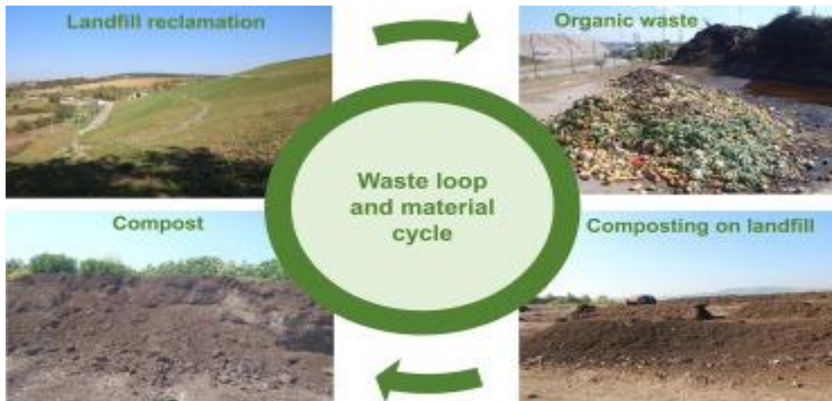
Figure 2. Alternative method of composting on a reclaimed municipal waste landfill in accordance with the circular economy (Vaverková et al., 2020)
