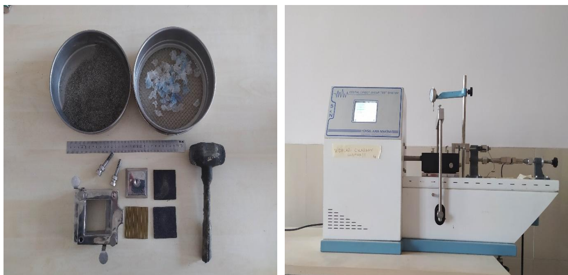
Figure 2. Preparation for direct shear test and experimentation
