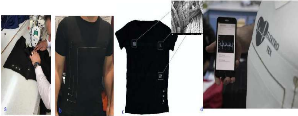
Figure 2. a) Placement of the sensors; b) External view of the smart garment; c) Interior of the smart garment and SEM image of the sensors; d) Electrical activity of the human heart transmitted to the smartphone via the ECG module.
