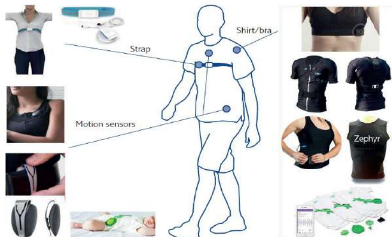
Figure 4. Position of some commercial wearable devices on the body that can predict ventilation from chest surface motion
