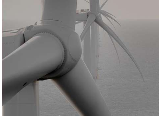
Figure 6.1. VESTAS V164-9.5 MW Wind Turbine [33]
